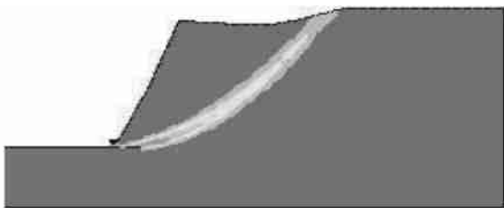
Fig.3 Continuous contours of horizontal displacement
